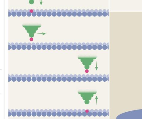
SPM can be used to move individual atoms. AFM is able to measure the atomic forces involved in these manipulations.
